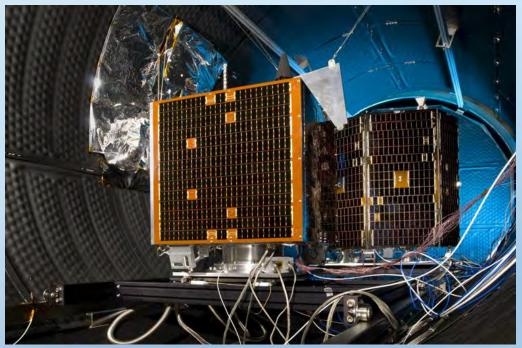
NX and NigeriaSat-2, the latest spacecraft manufactured for the National Space Research & Development Agency, under environmental testing at Rutherford Appleton Laboratory, Didcot, UK. Both satellites were manufactured at SSTL Guildford. *Picture courtesy of SSTL*
