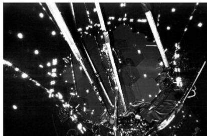
AOS Source Plate inward facing sources are used during the Field Alignment Test to measure ISIM to AOS Alignment
