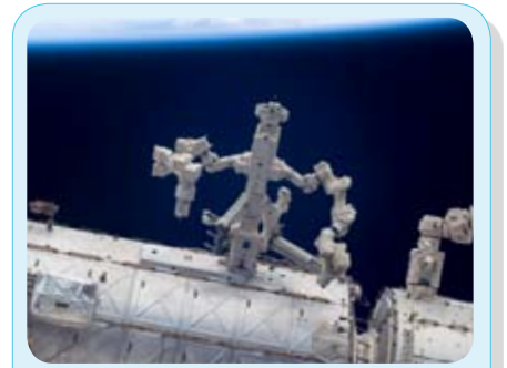
Dextre, the world’s most complex space robot, was built by the Canadian Space Agency for the ISS. Dextre has arms 3.35 meters (11 feet) in length and can use power tools as fingers.
