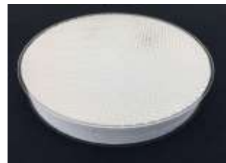
Mirror constructed with 3D Printed fused silica core
