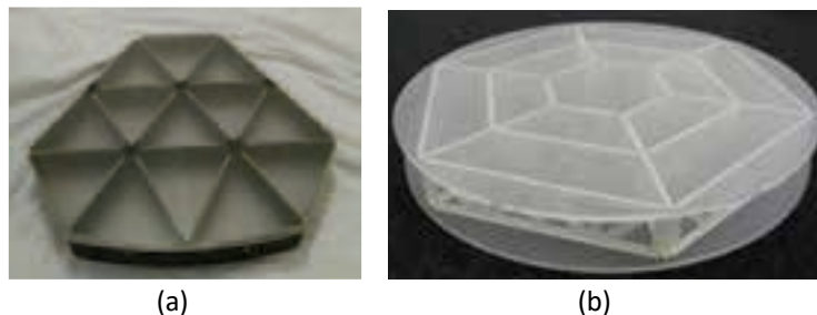
Figure 9: Examples of constructed core mirror technology: a) composite core and b) ULE ® core
