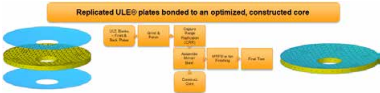
Figure 8: Constructed core process flow
