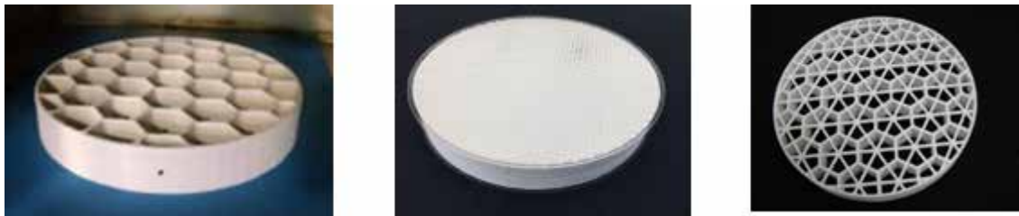
Figure 11: Examples of mirror cores made with additive manufacturing processes
