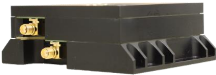
Exhibit 7: Innoflight cubesat format radio
