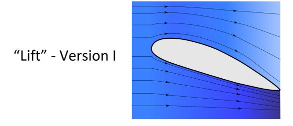
Movement of a wing through the air generates a pressure differential that "lifts" the wing.
