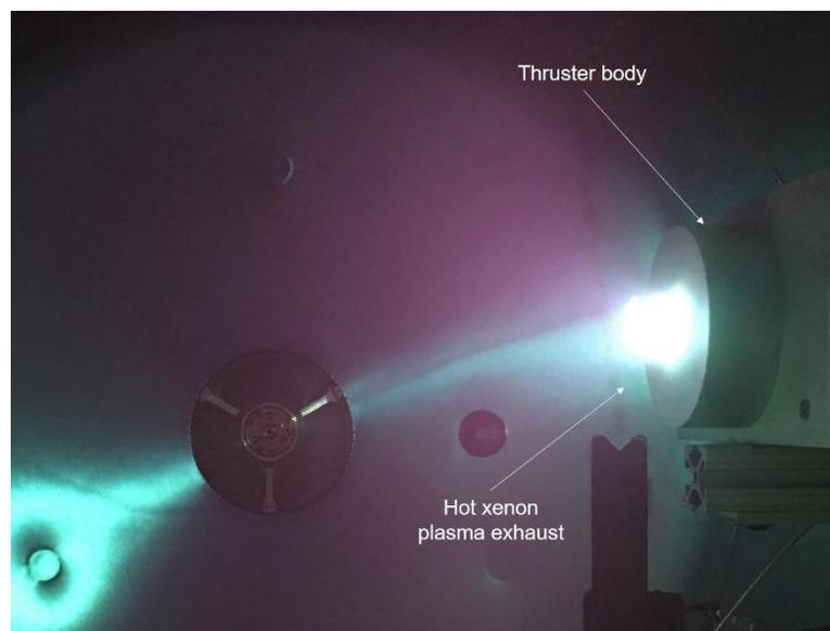
Figure 2: An image of the RFT-2 firing in the Phase Four laboratory.
