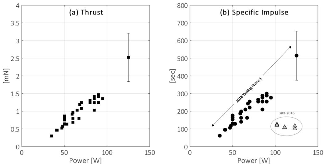
Figure 3: (a) The RFT-2 thrust measurements versus power and (b) measured specific impulse versus RF power between 40 W and 125 W at 0.5 mg/sec xenon mass flow rate. Data in gray show the previously presented results of The RFT-0 proof-of-concept system [5].
