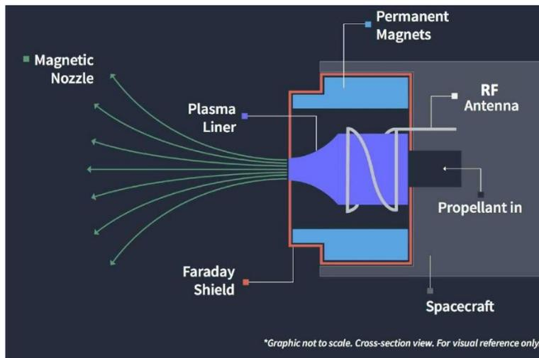
Figure 1: A diagram of the Phase Four RFT and critical internal components (not to scale).
