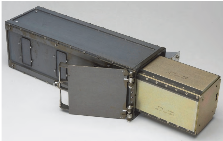
Figure 2. Photograph of a P-POD CubeSat deployer with a mock-up of a three-unit CubeSat. (NASA image)
